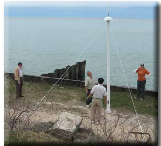
Setting up the radar transmitter antenna: (left to right) Calvin Teague (CODAR), Guy Meadows, Suwen Wang (CODAR), Amanda Mims.
